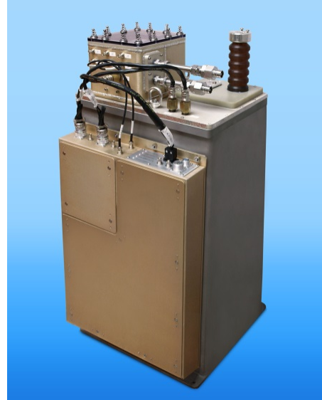
Figure 1. Solid-State Switch to Replace Thyatron.
