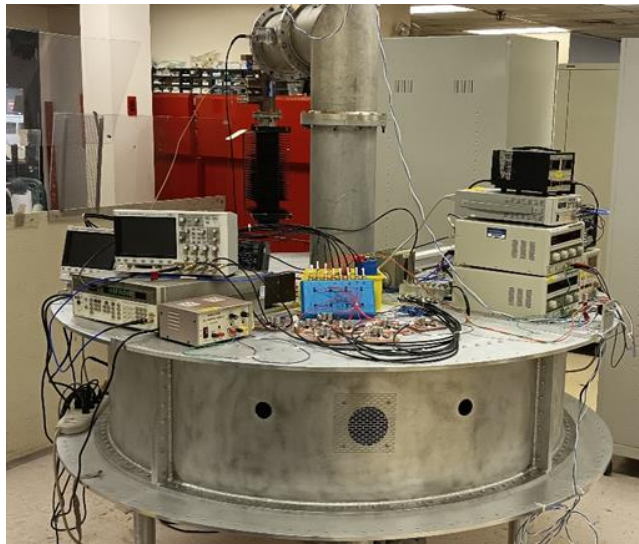
Fig. 1. Phase I full-scale 120 MHz Direct Cavity Combiner populated with 8 modules achieving 10 kW.
