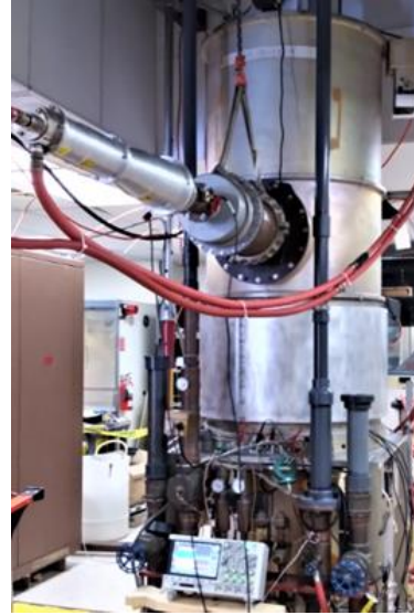
Fig. 3. FPA assembly at DTI with short pulse water load attached to front coaxial output.
