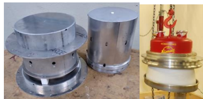
Fig. 1. (left) Surrogate tetrode made to the mechanical dimensions of the actual 4CM2500KG tetrode and the added resistances to emulate the electron beam currents (right) photo of 2.5 MW high power 4CM2500KG tetrode.
