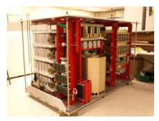
Fig. 6. Long pulse ILC Marx modulator in final stages of completion at DTI.
