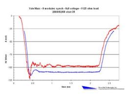
Fig. 4. A test pulse of the nine-stage (20%) short pulse Marx has initial charging voltage of 12.5 kV, resulting in 110 kV into 1125 ohms. (Lower/blue: voltage in kV; upper/red: current in amps).
