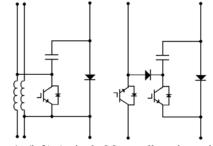
Fig. 1. (left) A single Marx cell, recharged via common mode choke, is suitable for short pulses. (right) Long pulses require prohibitively large choke cores, thus recharge is better served via a second switch.
