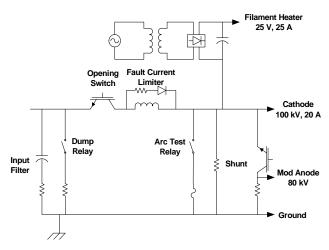
Figure 3. Solid-state switch schematic for the 100 kV, 100 A CW transmitter opening switch at the Advanced Photon Source.
