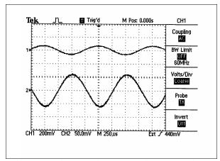
Figure 7. Linear voltage control. Top: 4 kV sinusoid in response to a signal generator sine wave input.
