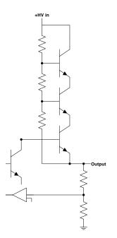
of the bottom IGBT; the phototransistor is driven by a fiber-optic cable. A sample voltage waveform is shown in Figure 8.
