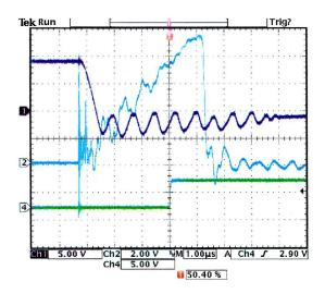
Figure 4. Opening switch arc response. Top trace: load voltage. Middle trace: load current. Bottom trace: switch control signal. The opening switch response time is 1.3µs after threshold crossing.
