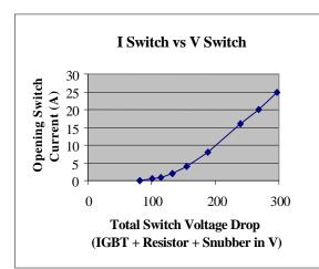
Figure 5. Voltage drop as a function of current in the 100 kV ANL switch. Efficiency at full current is 99.7%.
