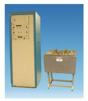
Figure 1. PEF pilot plant. Capacity up to 400 l/hr. Power electronics in cabinet on left; four-chamber processing unit on right.
