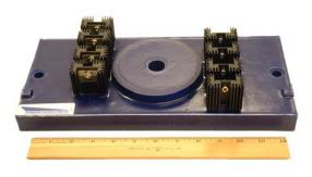
Figure 5. 20 kV, 100+ A, PPT switch module.
