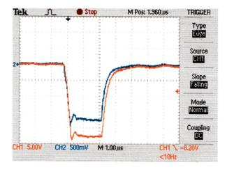
Figure 6. 20 kV, 35 A pulse into orange juice. Risetime ~ 200 ns, 1 kHz frequency
