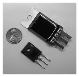
Figure 4. Pulse power transistor (PPT) top; conventional T0-247 bottom.
