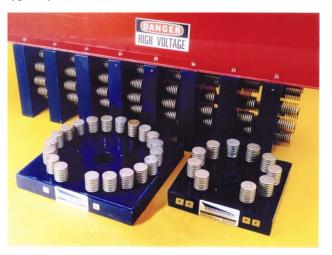
Figure 2. High voltage switch modules.
