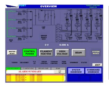
Figure 10. CJS PLC control screen. This is one example of a nested set of control screens, allowing the operator to view and control system operation. Multiple levels allow the operator to rapidly zoom from this overview of one group, to details of each elements' settings and performance.
