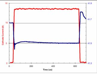
Figure 11. Cathode voltage and current pulse into a single TWT.
