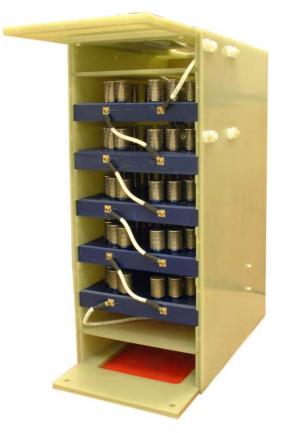
Figure 8. Solid state cathode switch assembly (modulator).
