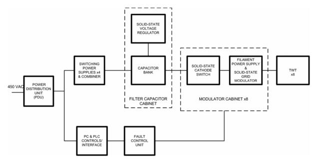
Figure 4. Block diagram of the new CJS transmitter. Diagram represents just one of two identical groups making up the transmitter.
