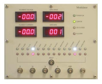
Figure 1. Modulator assembly fault control panel. Filament and grid voltage and current readings are displayed, along with system status and fault indicators. BNC outputs are provided for monitoring of time varying parameters within the modulator.
