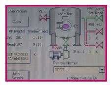
Siemens S7-200 Series "Touch Panel" Control Graphic Operational Display - Pass Word Protected
