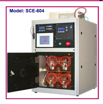
Anatech's multi chamber system allows plasma processing of up to four samples at one time while avoiding cross contamination.
