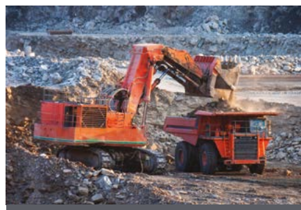
Tracked excavators (>100 tons)
