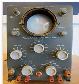
Oscilloscope with synchronized sweep. "HOR. SELECTOR" sets horizontal frequency range (the capacitor); "FREQ. VERNIER" adjusts the free-running frequency; "SYNC. AMPLITUDE" sets the gain to the comparator.
