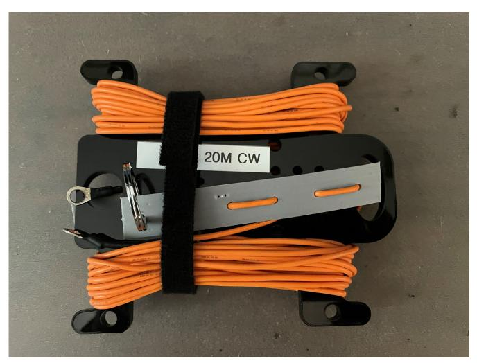
I used my resonant 20m dipole and added 3 extra radials, so I have 1 vertical element and 4 radials, all of same length. Achieved 1.2:1 SWR, no tuner needed.
