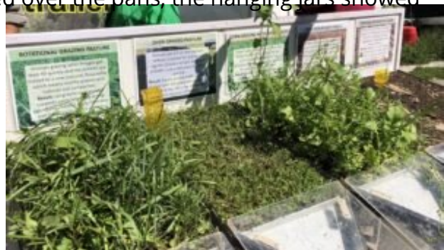
This soil simulator uses topsoil from a healthy and an overgrazed pasture, as well as sections of cornfields with cover crop, mulch cover and no cover. Livermore Falls Advertiser photo by Nicole Carter
