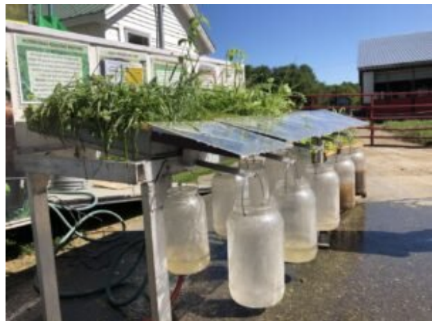
The soil simulator after an inch of water is sprayed over it, demonstrating how soil health impacts rainwater runoff. Livermore Falls Advertiser photo by Nicole Carter
