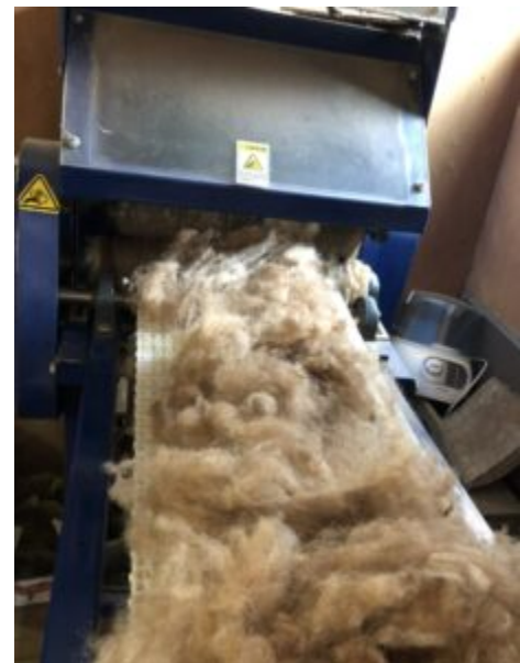
Once washed and air-dried, Harney feeds a sheep fleece into the “picker” which separates the fibers. Nicole Carter/Advertiser Democrat
