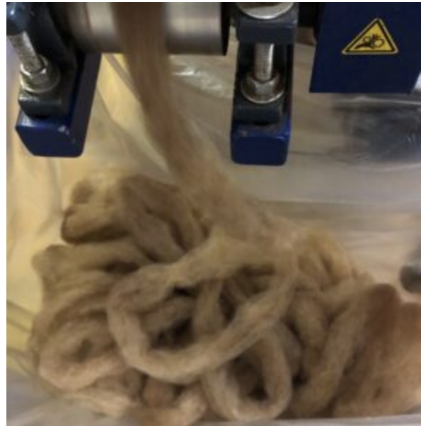
Carded fiber is fed into the “sliver” which pushes out finished roving, ready for hand spinning or other fiber arts. Nicole Carter/Advertiser Democrat
