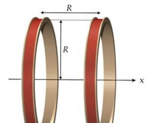
We designed paired electromagnet sets, Helmholtz Coils, to minimize 2 largest field components
