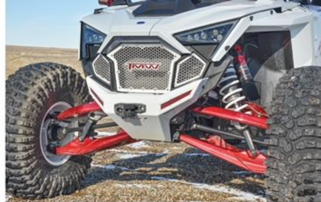
TMW helped finish off and protected the front end of this machine. That bumper hides a Warn winch outfitted with a Factor 55 flat hook. The Glossy White/Diablo Red powdercoat really changes the look of this machine, thanks to Coating Plus in Boise, Idaho.
