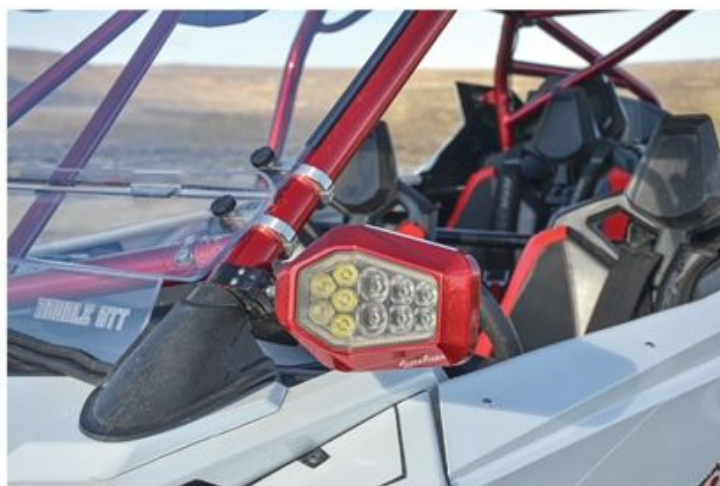
Sector Seven's latest product is a two-zone lighted mirror with running lights, signal markers and a convex lens that can be adjusted separately. Furthermore, the accent lighting can be controlled with a smartphone app.
