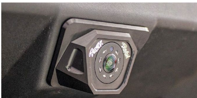
Polaris has the option for a backup camera across all models. For the Pro R, the area they mount it to is blocked by part of the cargo box. Part of that box appears in the screen. The Sector Seven mount moves the lens out slightly, expanding the view with no blockage.
