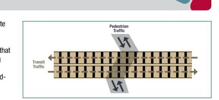
Figure 18: Z-Crossing Schematic
