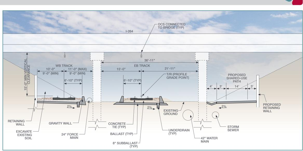
Figure 19: HRTs current typical section design under Interstate 264
