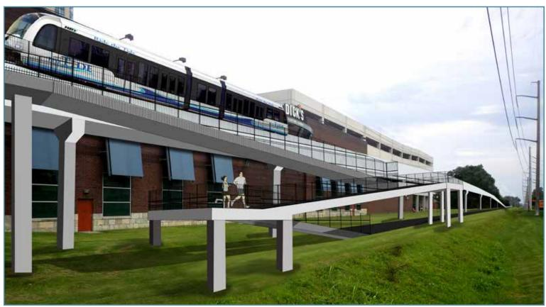
Figure 21 : Layout of Pedestrian Crossing Over Independence Boulevard with Ramp to Market Street (for conceptual purposes only)
