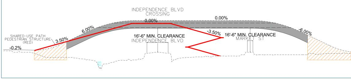
Figure 20: Profile of Pedestrian Crossing Over Independence Boulevard
