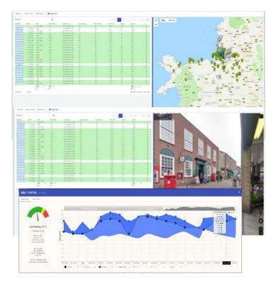
All the information can be drilled down and audited, standard information includes high temperature, current temperature, ambient temperature, minimum temperature. All data is fully searchable and integral to Google maps to provide exact substation location.
