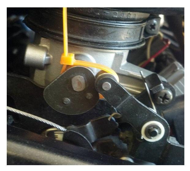
The last step is to keep the secondary shaft from rotating. Shown below with the pink zip-tie, the important factor is to go underneath the spindle for the high idle cam arm. This zip-tie does not need to be very tight. It's only purpose is to keep the cam from rotating clockwise. The orange tie and follower are preventing it from rotating counterclockwise.
