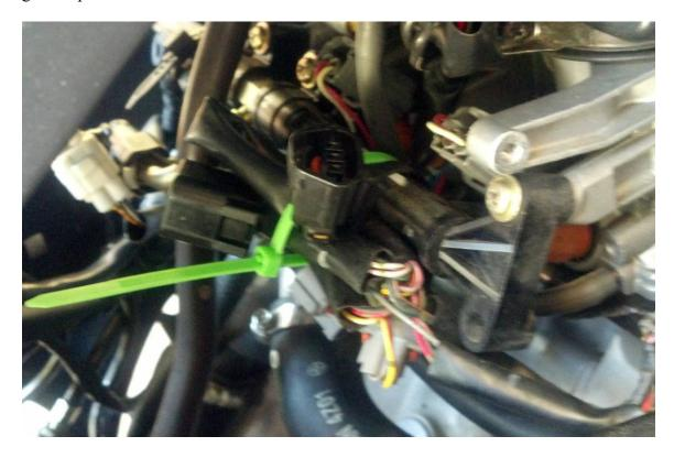
Next, on the left side of the bike, a smaller zip-tie is used to hold the high idle cam completely shut. A smaller zip-tie is used here because it will grip the groove in the cam follower and prevent it from sliding off. Note the position of the cam. This position is not possible with the STVA installed, but is critical to this procedure. This zip-tie needs to be fairly tight. This is shown with the bright orange zip tie.
