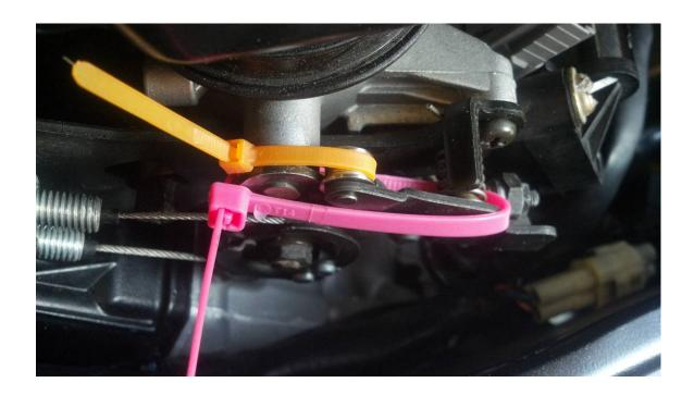
There are other methods available to complete this task. As long as the high idle system is held shut, the cam is secured from rotating, and the method of securing it is done outside the airbox, it will work. Below are two examples of the cam being secured with safety wire.
