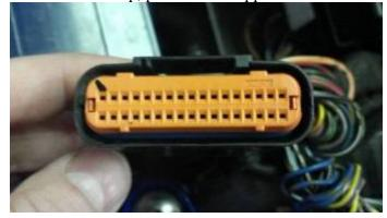
3) Small sewing pins in the gator clips of a digital multi-meter make excellent probes. Be gentle when inserting them as not to deform the socket in any way. One circuit of the stepper motor is pin #1 to pin #18. #18 is the first pin in the second row. Below shows a good circuit reading 6.8 Ohms of resistance.
