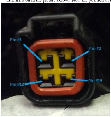
2) In similar manner to phase one, you will test for resistance between the STVA connector and the ECU connector. Be below pictures show a good test for pin #1 with a reading of 0.03 Ohms.
