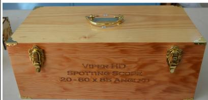
thick. Top front, rear and ends are mitred joints. While the bottom is made from 8mm plywood rebated. The lid was cut off after assembly with Titebond 3 glue.
