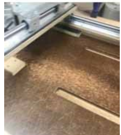
Sled with dust extractor, ie, very little, if any, dust.
