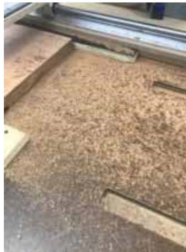
Sled without use of dust extractor, ie, lots of dust.
