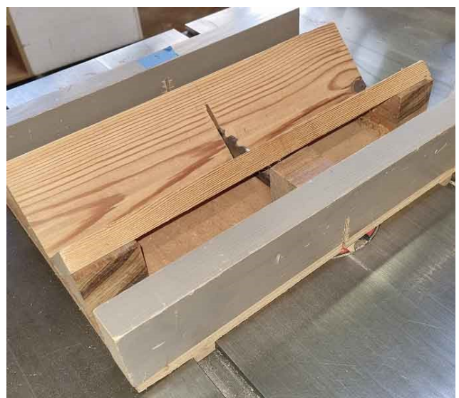
Front view of Mitre Spline Jig.. Note one of the Guide Rails running in the Mitre Gauge slot on the table.
