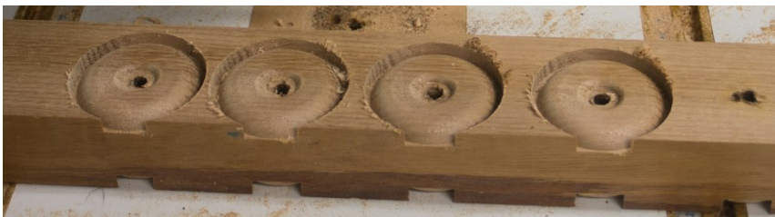
Circles cut half way through, ready to be turned over for the second pass
