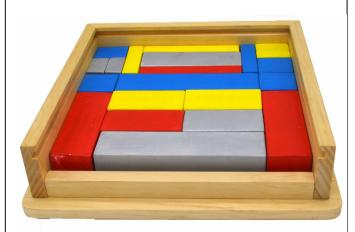
The box is made with mitred corners with shallow dados on the inside surface to allow the puzzle cover to slide in. The puzzle pieces need to made to precise sizes that are explained in the drawings. I have painted each block in very vibrant colours using water based acrylic colours purchased from Meeden Art Supply Co., Ltd . via Amazon.
