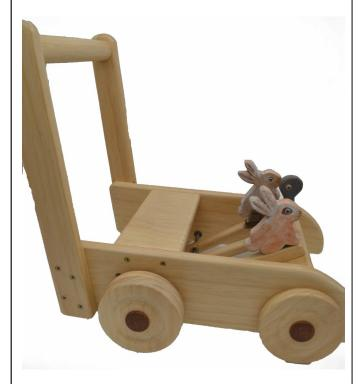
The choice of animal is endless and I decided to relive the great race between the hare and the tortoise. The moving mechanism is quite simple. Each animal is sitting on a square stick threaded through a metal rod at the other end. The rear axle has a number protruding dowels above the square sticks. As the rear wheels and axle turn the dowels push down on the sticks causing the pivot action. Result of this race is same as in history. The hare won by half a head.
