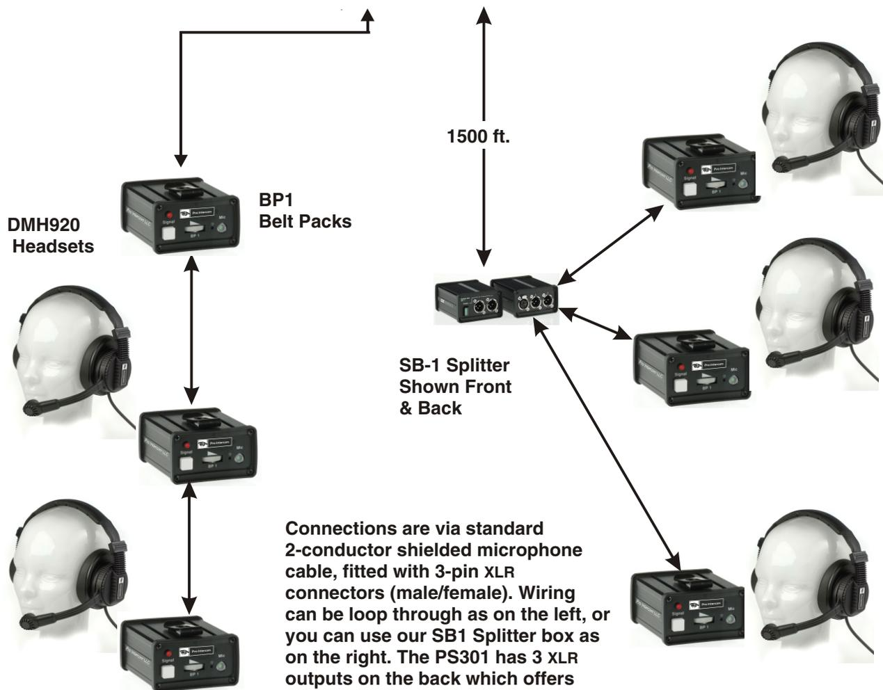
Connections are via standard 2-conductor shielded microphone cable, fitted with 3-pin XLR connectors (male/female). Wiring can be loop through as on the left, or you can use our SB1 Splitter box as on the right. The PS301 has 3 XLR outputs on the back which offers more wiring flexibility. The PS301 is capable of driving 66 belt packs and the distance being dealt with is not a problem.
