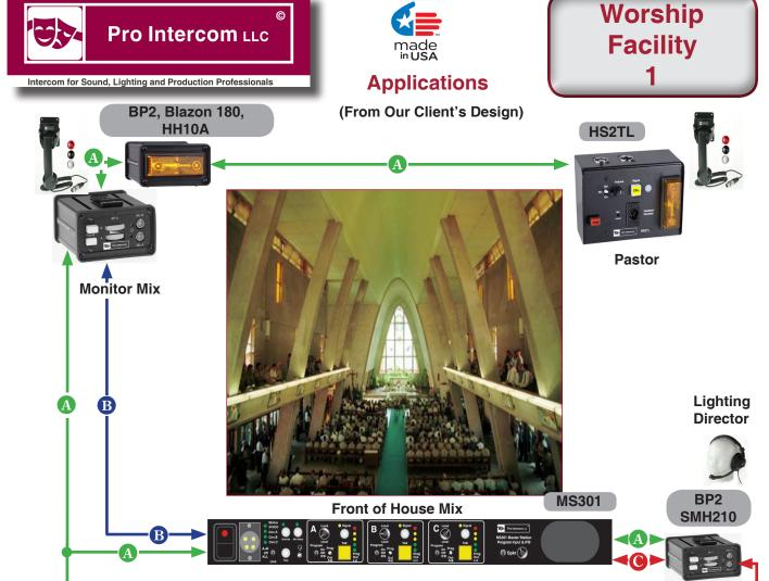
In this system, the power and main control are provided by an MS301 Master Station. The F.O.H. Mix position
