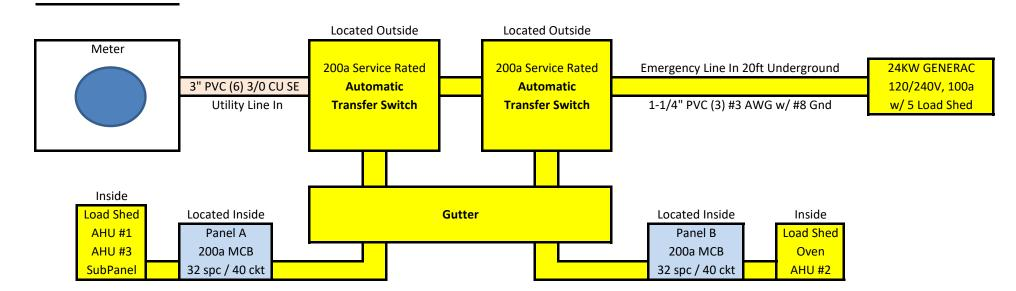
New 24Kw Generac Generator w/ 2-ATS's and 5 Load Shed Circuits each
