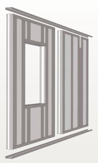
Example shows typical window rough opening, beam pocket, and top and bottom track.
