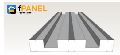
**fPanel** - 48" Max width, 144" max length. Panels connect end-to-end and side-to-side for coverage. Rebar troughs to form grade beams, top with rebar mesh and 3-4" concrete. Panels connect end to end and side to side for coverage.
