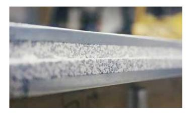
**Insect Deterrent** - Uses steel and expanded polystyrene - neither of which are of nutritional value to wood-boring insects such as termites.
