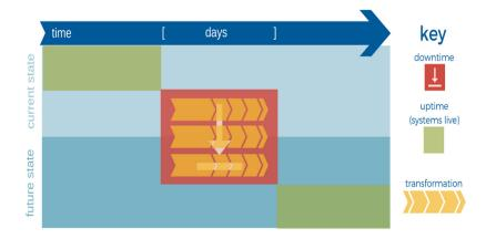
In this illustration, the production system continues running while the data transfer and replication and the transformation process occur simultaneously. Near Zero Downtime replicates data changes every hour, instead of requiring a full snapshot while production systems are down. Since the primary data and replication take place during uptime, only a small dataset is left to synchronize during downtime – which can be done with high speed.
