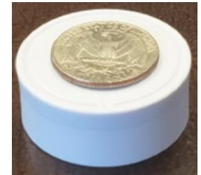
The white BLE Beacon is slightly larger than a U.S. quarter
