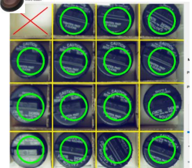
PC screen shot shows 1 slot missing a part. Container label won't print until slot is filled.
