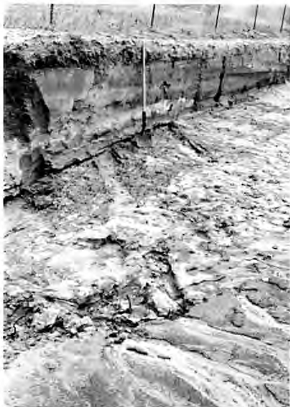
Figure 4. Ruts on the surface of buried soil beneath levee (shovel standing between the ruts is 1.5 meters [4.8 ft.] tall). Note the bedded nature of the levee fill and near absence of soil development at the modern surface.
