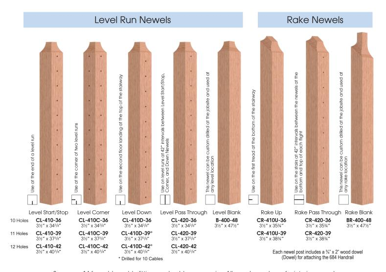
See page 14 for cable, cable fittings and cable accessories. All wood newels are for interior use only. IMPORTANT: Our Wood Newels above and Cable System is designd for stairways with 7-1/2" rise and 10" run (approx. 36.9°)
