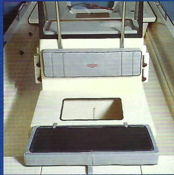
CONSOLE WET BOX
