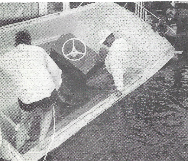
ramp test With drain plugs pulled.
