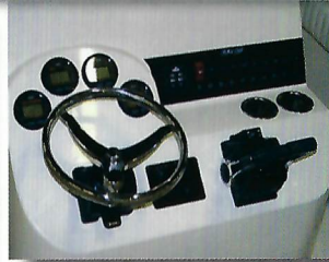
ERGONOMIC DASH WITH HYDRAULIC STEERING
