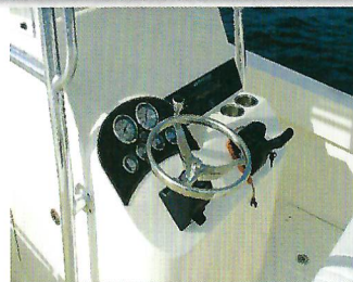
CONSOLE WITH HYDRAULIC TILT STEERING
