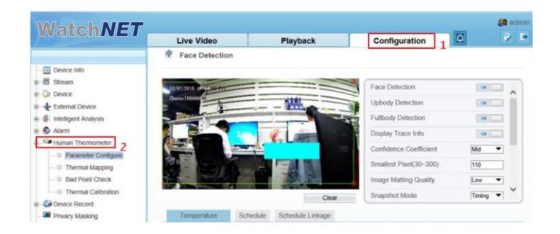
1. Parameter configuration interface: Configuration(Mark 1)->Human Thermometer(Mark 2).
