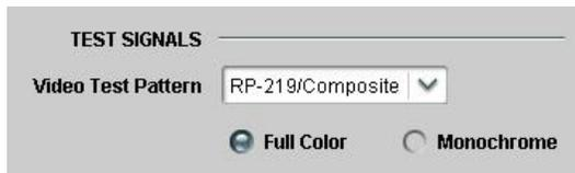
Use the radio buttons to choose if the test pattern is to be displayed as *Full Color*, or *Monochrome*.
