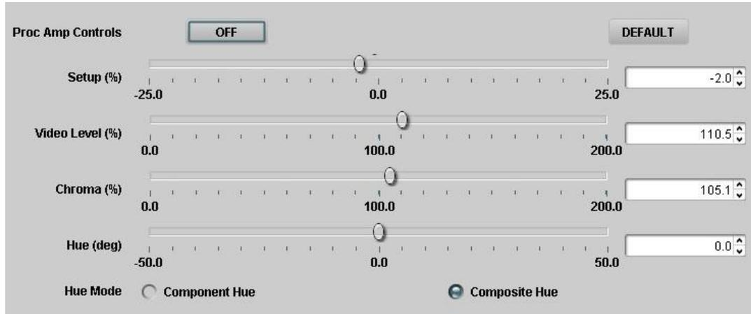
The **Proc Amp Controls** button is used to enable or disable all four Proc Amp controls. When set to **ON**, the Proc Amp controls are active. When set to **OFF**, the Proc Amp controls are bypassed (unity gain) and any control settings are ignored.
