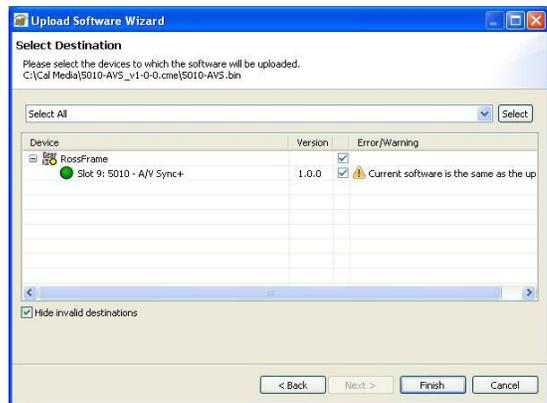
5. Click **Finish** to begin installing the new firmware. When the installation is complete Click **OK**. The Upload Wizard will close and the 5010-AVS will automatically reboot with the new firmware. Verify that the new version numbers are displayed on the Dashboard™ control *Product* menu.
