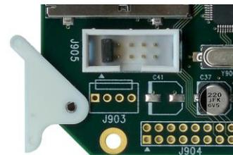
Figure 4-2 Boot-Loader jumper location
