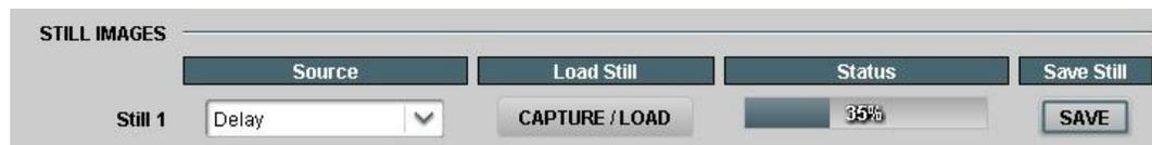
The Status bar shows the progress of the still image file being saved, and will display 100% when the image file is completely saved.
