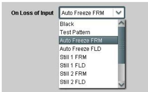
Use the *On Loss of Input* drop-down control to select the default video source.
