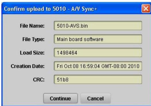
5. Click **Continue** to begin installing the new firmware. When the installation is complete the 5010-AVS will automatically reboot with the new firmware. Verify that the new version numbers are displayed on the Dashboard™ control *Product* menu.
