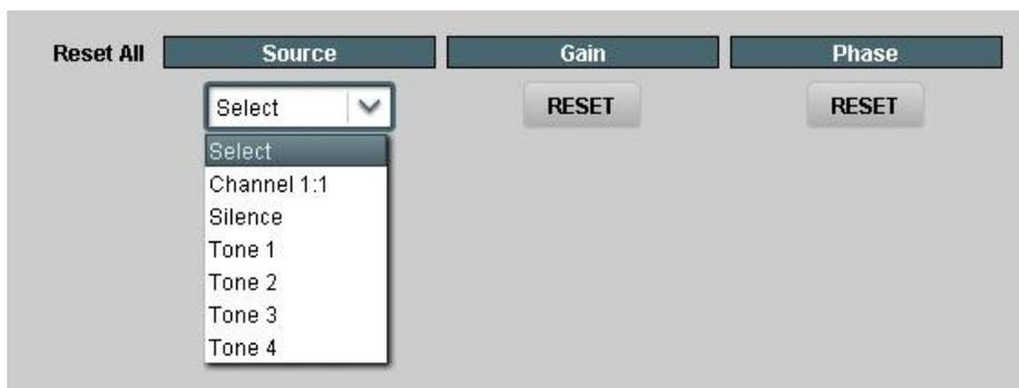
The **Source** selection under **Reset All** is used to quickly assign all 20 channels to the selected source.
