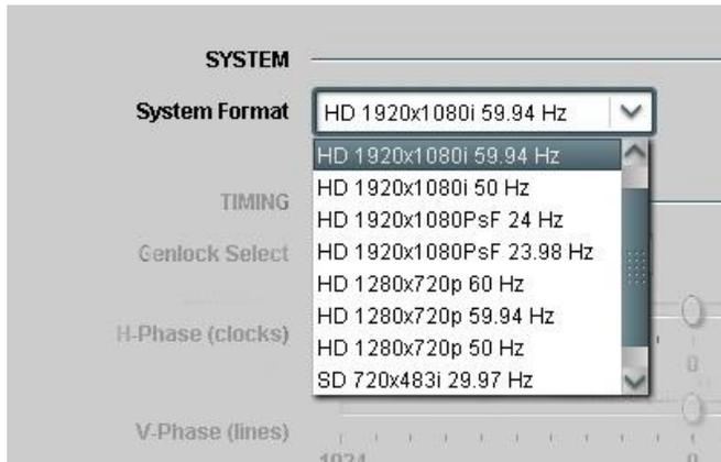
Use the *System Format* drop-down control to select the video format for the 5010-AVS. The operator may choose from a list of standard formats and frame rates.
