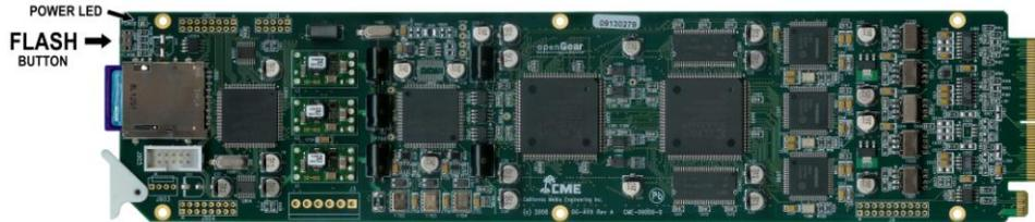
Figure 4-1. FLASH button and POWER LED location.
