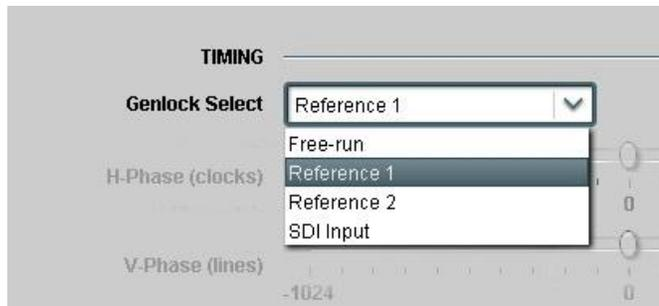
The following controls adjust the timing of the video frame synchronizers. Because of internal processing delays (approx. 3+ lines), a phase setting of zero clocks / zero lines will guarantee one frame of delay in the synchronizer.
