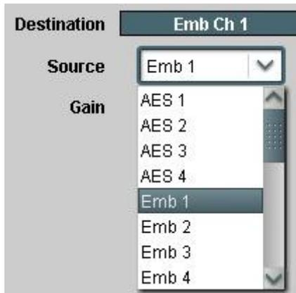
The choices include AES input channels 1 through 4, Embedded input channels 1 through 16, Audio Test Tones 1 through 4, and Silence.
