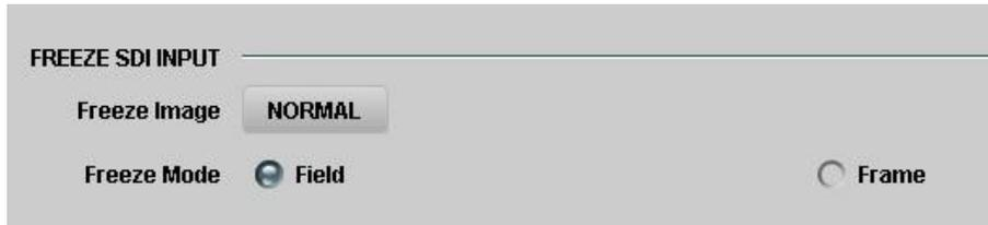
The **Freeze Mode** setting allows the frozen image to be displayed as a single field or a full frame.
