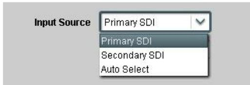
Use the *Input Source* drop-down control to select the SDI source for both video and embedded audio.
