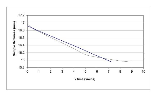
Corrected zero value = 16.9 mm  $\sqrt{t_{90}}$  value (read from plot) = 6.7 mins
