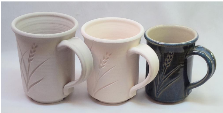
This image shows a mug that has dried, a bisque fired piece, and a mug that has been glazed and fired again.
