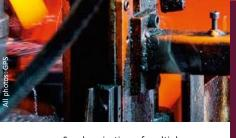
Synchronization of multiple servo axes of an IS machine in the microand millisecond range.
