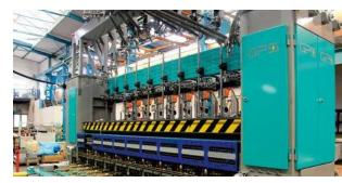
IS machine for the production of bottles and jars in all shapes and sizes.
