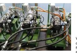
Unlike conventional valve hydraulics, the servo pump directly transmits the energy from the drive motor to the hydraulic press cylinder. In other words, the servomotors provide only the energy that is needed for each phase of the press process. Precision, compactness, low maintenance expenses, and outstanding energy efficiency are all the encouragement Waltec needs to go fully electric by converting the last of its nonelectric drives.
