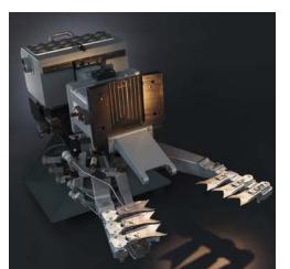
The Simotion-based Heye servo drive controls a plunger (above), dual-motor shears (left), and other hot-end components quickly and precisely.
