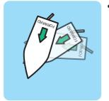
Note: If you turned to the right on engaging reverse gear, the prop effect, coupled with the current, would bring the stern of the boat back to where it started.
