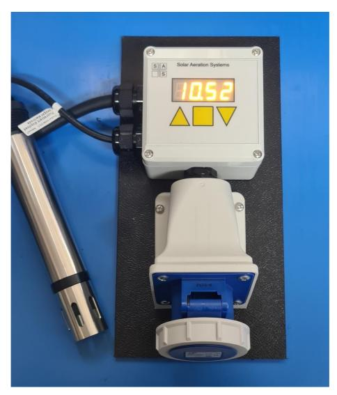
The DO5021 optical probe is supplied with 8 mtrs cable as standard but can be increased with connectors or single length at the factory.
