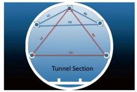
The installed prisms are then connected by lines and creating 2 triangles RAPID Convergence calculates the measurement between the connecting lines of the prisms
