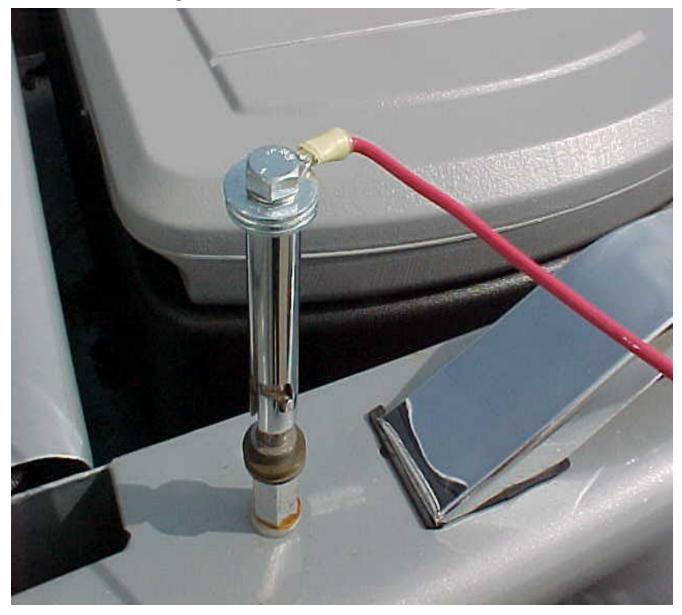
This is one of the one-piece 3/8x24 single-hole-to-SO-239 mounts (solid brass center pin, no pressed fitting).
