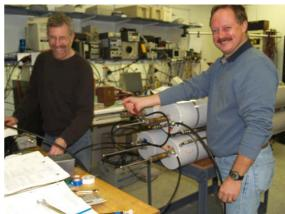
spent a whole Saturday testing everything and going through the various steps to tune. The duplexer system consists of 4 cans, two on the receive side and two on the transmit side. Each can acts as a very narrow high Q band pass filter as well as a notch filter. On the transmit side the band pass is set to the
