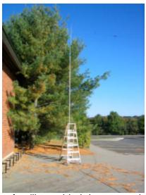
and the feedline guided down over the "tower" and into the building. The rig, which could handle VHF and HF, operated on battery as well as A/C. Unpack-to-setup was less than 45 minutes The station enabled reliable communication with other area EOCs in the SET and served as a good test of an "in-the-field" emergency "go-kit".
