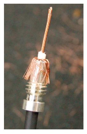
One particular problem I have is with the shield on RG-174, the silver plated stuff anyway. With regular solder, even with high heat the solder wouldn't stick well and often the insulation melted to the point of damage.
