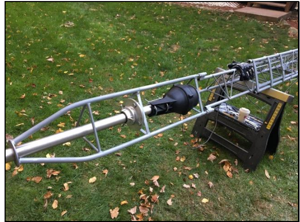
New thrust bearing with rotator and mast installed.
