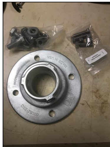
DX Engineering tower thrust bearing
