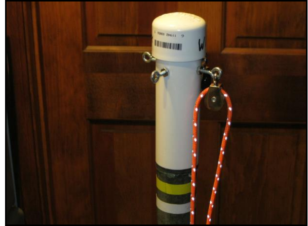
Mast adapter for lifting wire antennas Photo Credit: W1QK
