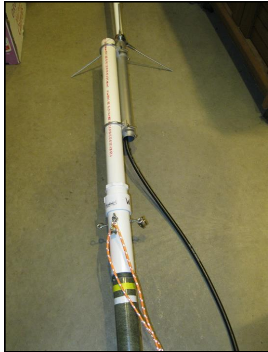
Mast adapter for raising wire antennas and supporting Dual-Bander antenna Photo Credit: W1QK -----
